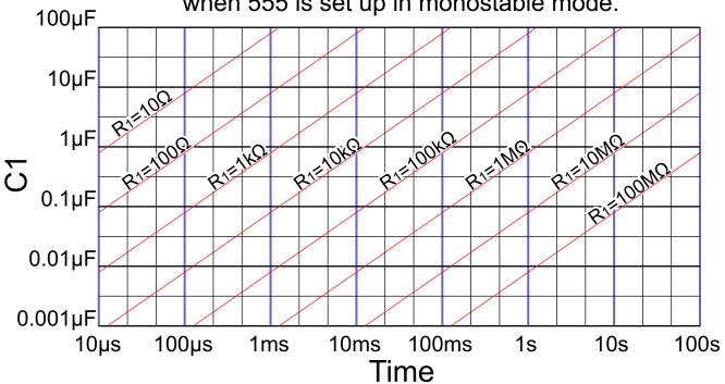
The time is calculated **t=1.1 X R1 X C1**. R1 is in ohms, C1 is in *Farads*. Example: If R1=100k and C1=100 $\mu$ F, 1.1 X 100,000 X 0.0001 = 11 seconds.
