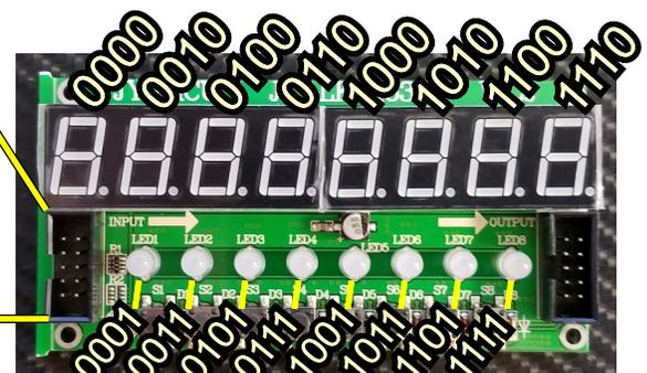
On boards with bi-coloured LED's, the addressing is exactly the same, though the board layout may be different.
