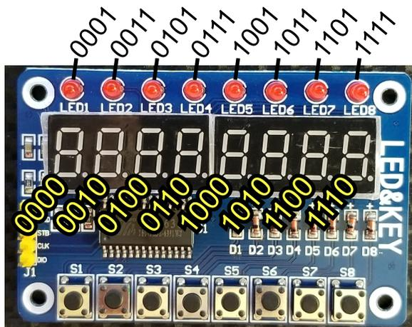
Addresses shown are the lower nibble required for display instructions. The upper nibble sets the addressing mode, the lower nibble dictates where the data byte should go.
